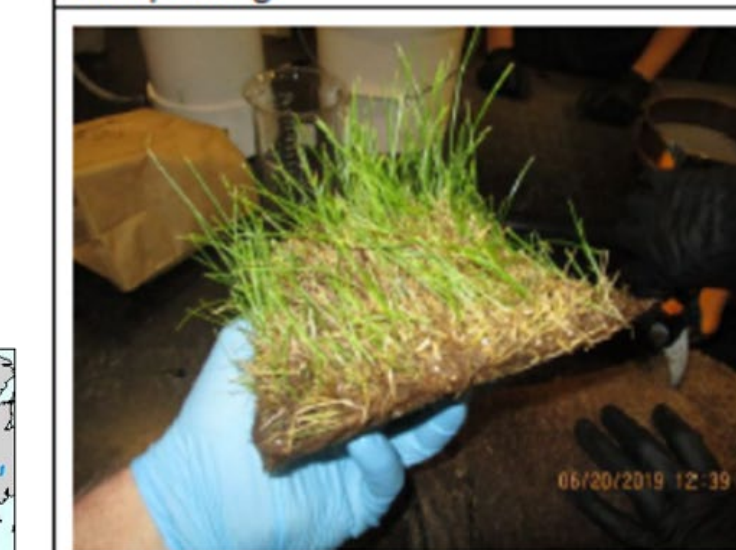
Figure 3. Thatch easily removed from sand support media at the test completion.
