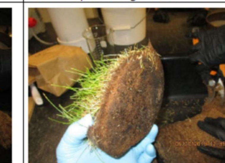
Figure 4. Thatch removed at test completion; with no evident sand from the support media.
