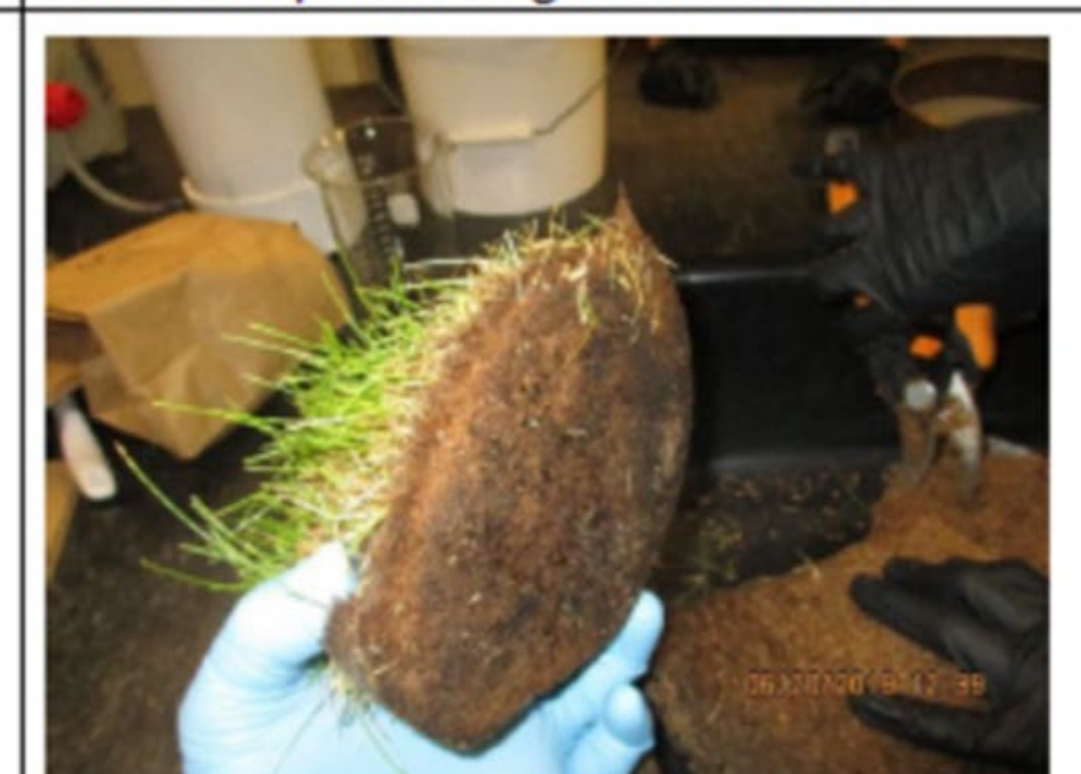
Figure 4. Thatch removed at test completion; with no evident sand from the support media.
