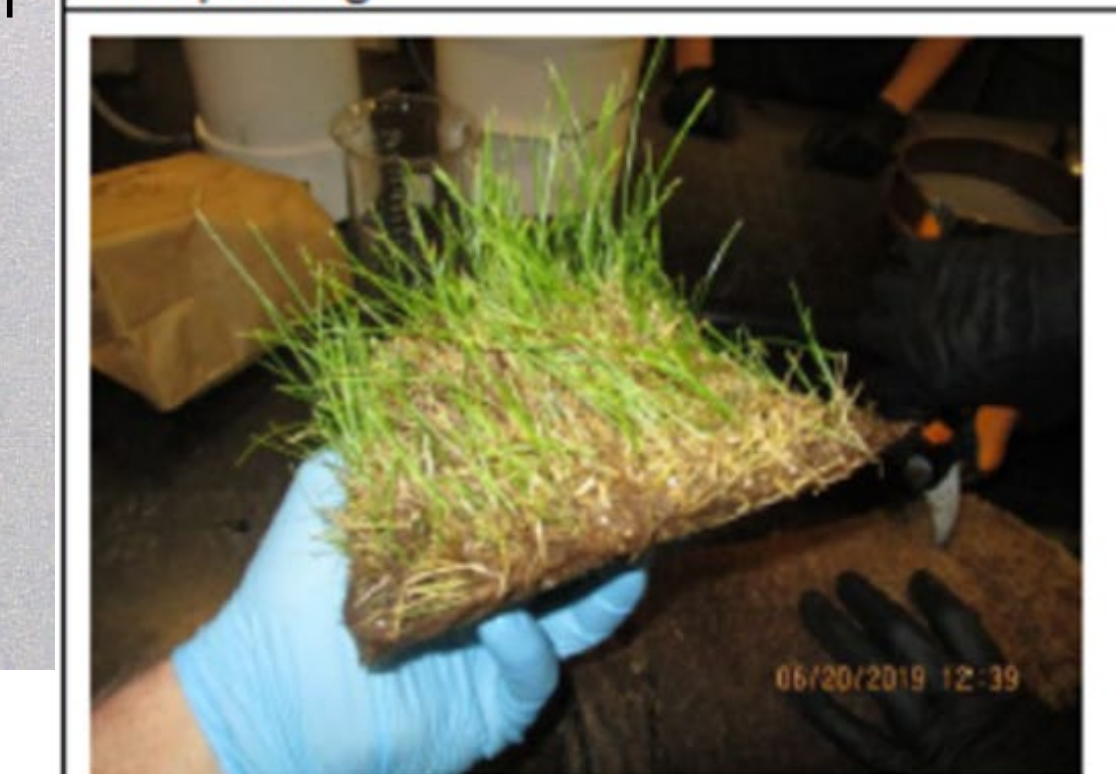
Figure 3. Thatch easily removed from sand support media at the test completion.
